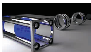
The MOTion. A linear radio frequency ion trap is co-located with a Ca magneto-optical trap. A time-of-flight mass spectrometer is radially integrated for ion identification.
