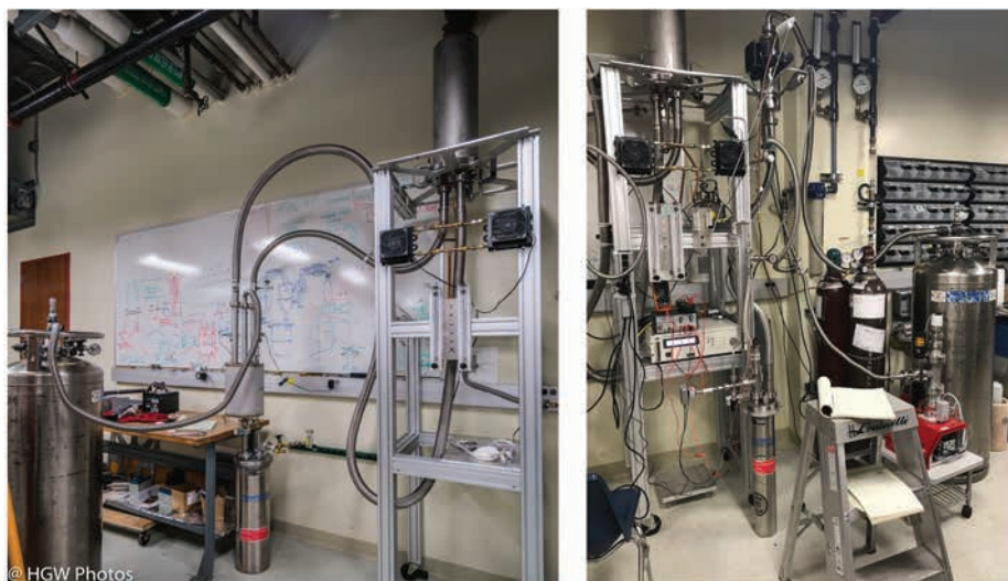
Figure 2. Left: Picture of the full-size prototype of liquid argon condenser for DarkSide-20k and the testing setup maximally simulating the operation condition of the real cryogenics system. Right: Picture of the stand-alone liquid argon system that can be used for various tests.
