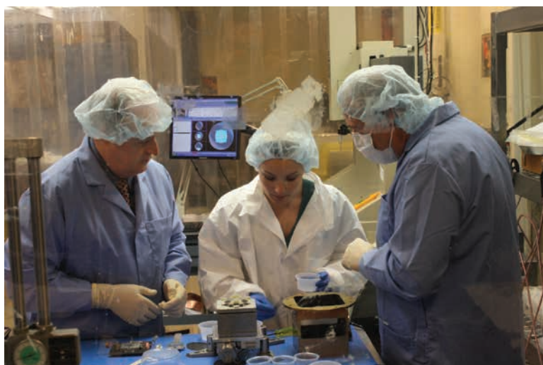
Professor McLean (left) with former UCLA Ph.D. student Kristen Kulas and Machinist Ted Aliado. They are assembling the very delicate detector system for the MOSFIRE spectrograph.
