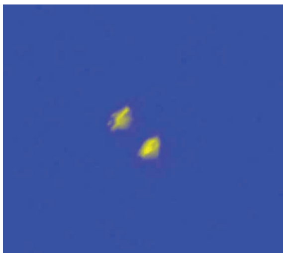
Best Friends. Two ^{133}\text{Ba}^+ ions being simultaneously laser-cooled in an ion trap. By coupling their internal state qubits to the collective motion of both ions, quantum computations can be performed using the phonons as a quantum data bus between qubits.
