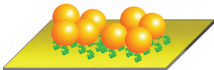
Fig. 3. Geometry of the nano-rheology setup, where gold nanoparticles (GNPs) tether the enzyme to a gold surface. The GNPs are driven by an electric field, while the displacement is read optically.
