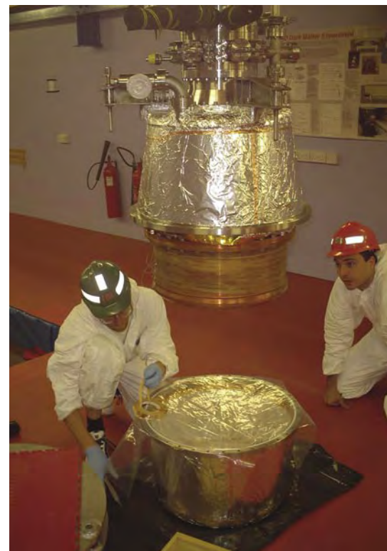
The ZEPLIN II, the largest discriminating detector in the world, was recently moved underground to the Boulby mine (4,000ft deep) to start the search for dark matter.
