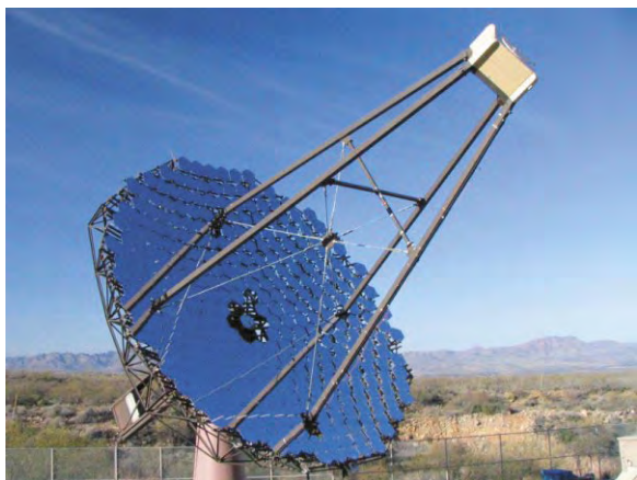
VERITAS (Very Energetic Radiation Imaging Telescope Array System) is a major new ground-based gamma-ray observatory with an array of four 12m optical reflectors for gamma-ray astronomy in the GeV - TeV energy range
