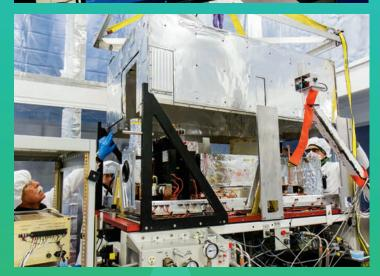
Above: A new isolated optical plate was built to hold our test cryostat (gold) and Zygo interferometer adjacent to our Coordinate Measuring Machine (CMM). This setup will be used to evaluate alignment procedures for the optical systems employed by IRIS.
